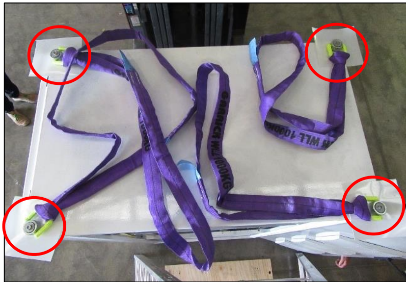
Figure 7: View of lifting slings attached to the unit
